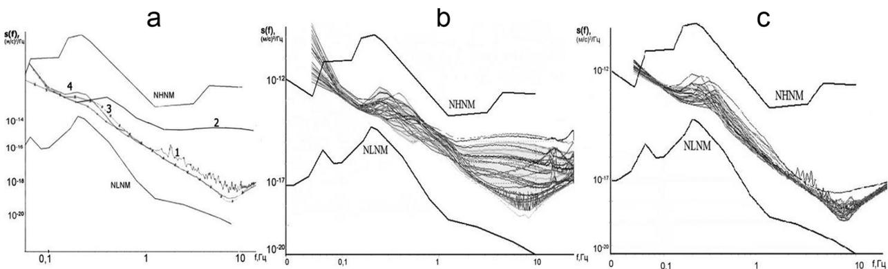
**Fig. 3.** Comparison of the daily power microseismic spectra of SVZ station for different months of 2017 with a generalisation by Peterson models: **a** – NLNM and NHNM – low and high microseismic noise models, respectively; 1 – May, 2 – August, 3 – October; 4 – December; **b** – diurnal power microseismic spectra in August; **c** – daily power microseismic spectra in October
